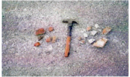
Figure 7. Some of the samples that were collected. On the left is some clay, and on the right is quartz. The hammer is included for scale. Photograph by Scott Little.
